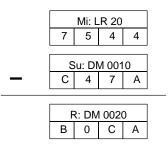
In the case shown below, -30,000 - 3,000 = -33,000 (8AD0 - 0BB8 = 7F18). The UF flag would be turned ON to indicate that this result is below the lower limit of 16-bit signed binary data range. (In other words, the result is a negative number below -32,768 (8000), not a positive number expressed as signed binary data.)
